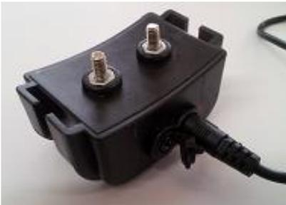
3) Install the strap to the collar by inserting them through the 2 brackets on the collar. Adjust the length and snug fit the collar to your dog's neck.
