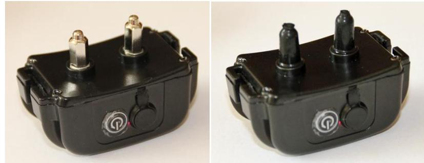
4) Test the shock of the collars by using the wire shock tester. Wrap the wires around the 2 metal posts of the collar then press the shock button. The bulb will light up if the collar is giving a shock.
